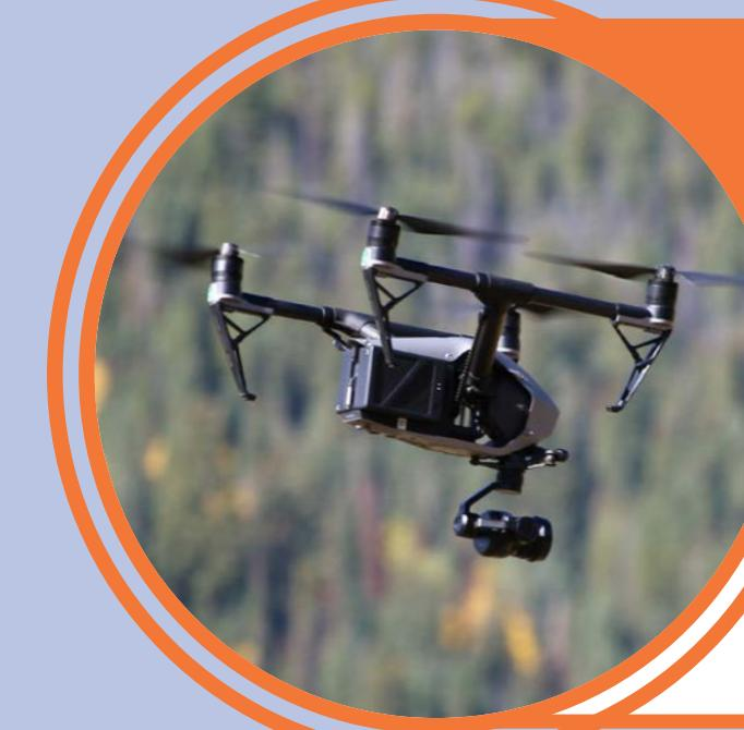
Quickly deploy unmanned aerial systems that take measurements and pictures of a crash to expedite crash investigations. Can also be used for ongoing traffic and incident monitoring.
