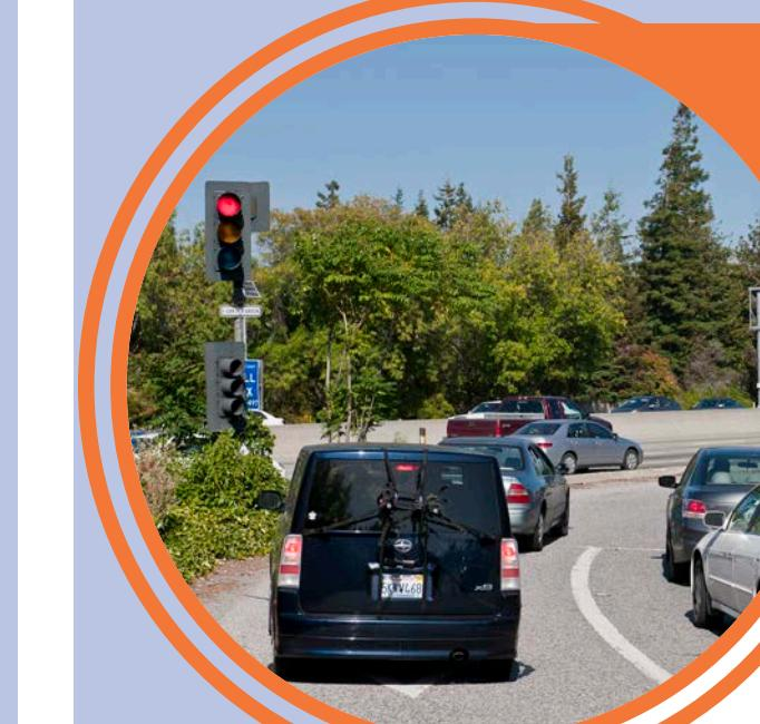
Meter traffic on ramps merging on to freeways to ease traffic congestion.
